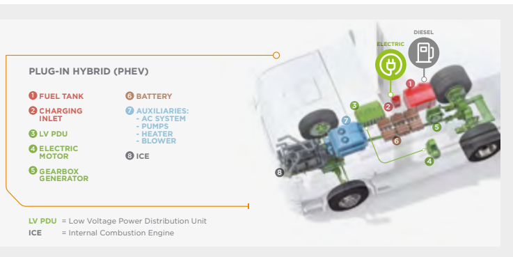
Figure 2: Typical Plug-In Hybrid (PHEV) Architecture
