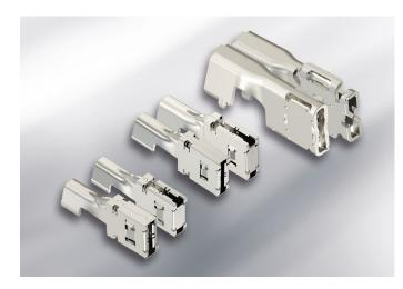
The new line of terminals, PCON 12, PCON 18 and PCON 21, have a common body design optimized for maximum vibration resistance while minimizing mating forces. Each is available with 90° and 180° mating directions and accommodates wire sizes ranging from 5 mm<sup>2</sup> to 95 mm<sup>2</sup> supporting continuous currents up to 400 Amps.
